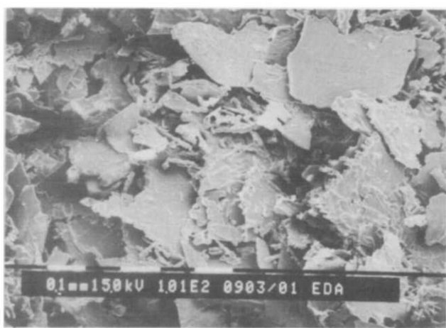
Figure 5 SEM photograph of the pure EDA ammonium salt prepared in the blank test
